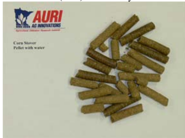
Figure 6- Corn stover with water (16%) – variability noticed in color prior to die plug
