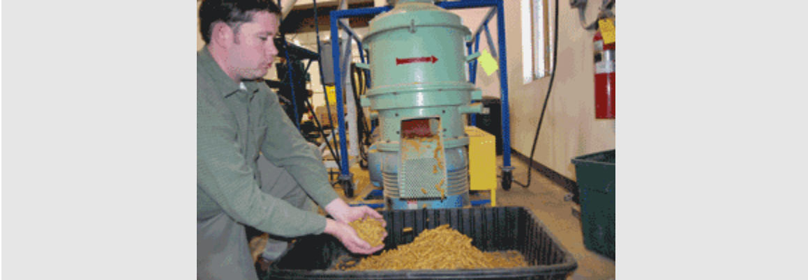
Kyle Cruit, director of sales and marketing for Hi-Tech Agro Projects Pvt. Ltd., examines distillers dried grains with solubles pellets produced by the company's PL500 flat-die pellet mill./PHOTO: RYAN C. CHRISTIANSEN, BBI INTERNATIONAL.
